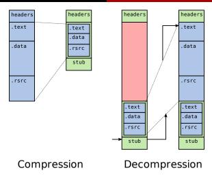
Figure: How runtime packers work
