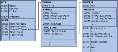
Figure: Identifying the current process in Windows (XP)
