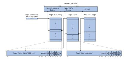
Figure: Paging on the x86 architecture
