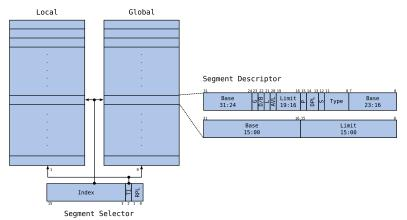
Figure: Segmentation on the x86 architecture
